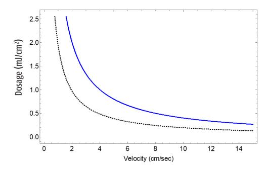
The upper, blue curve is the "near" radius, corresponding to the inner CPAP tube surface being directly adjacent to the outer quartz tube on the Bullet, and the lower, dashed black curve is the "far" radius, corresponding to the farthest possible distance from the Bullet LED to the inner surface of the CPAP tube.
