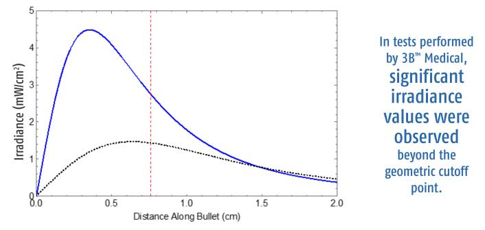
The results shown in the plot indicate that there is a distance of about 0.5 cm along the CPAP tube where there is an irradiance of at least 1 mW/cm<sup>2</sup>, with the potential for a much higher irradiance depending on the relative orientation of the Bullet and the tube.
