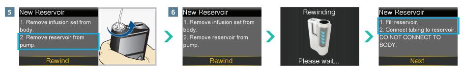
Remove the used reservoir from the pump.
