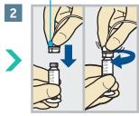
Gently push the tubing connector onto reservoir. Turn clockwise until locked. You will hear a click.
