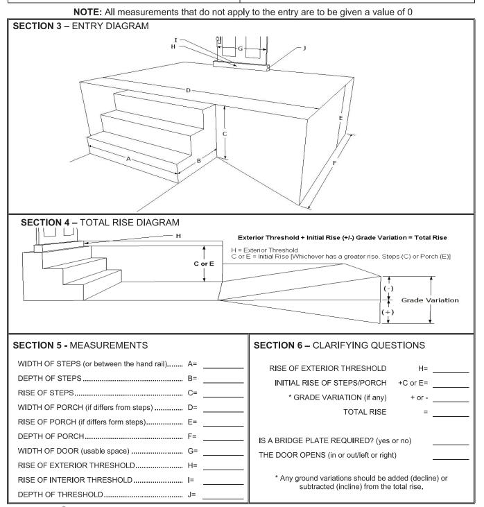
EZ-ACCESS<sup>®</sup>, along with most regulatory agencies, recommends 1-foot of ramp run per 1-inch of rise in height (1:12 ratio). For example, if a porch and steps have a total rise of 20-inches, a ramp with a 20-foot run would be required. Please note that this does not include platforms that may be necessary for the ramp system.
