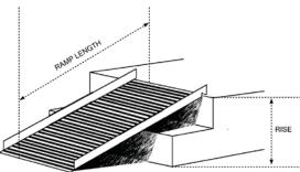
**B)** Once this height is determined, (i.e., 40" rise), measure out 40' to see if there are additional drops or difference in rise due to uneven yard, etc.
