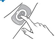
NOTE: You cannot turn the gel pad units on by pressing the remote control. Press the + button on the gel pad unit to turn the device on.
