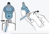
Change 2 AA alkaline batteries when begins to flash on the display.
