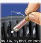
6. Activate (crush) processed indicator by inserting into the incubator.
