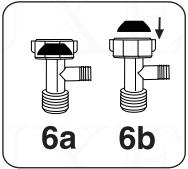
6a: Make sure that there is a black rubber washer inserted at the top of the t-adapter.6b: If it is not already there, insert it as shown in figure 6b.
