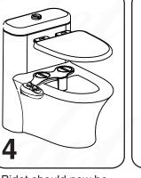
Bidet should now be aligned with the coupling holes.
