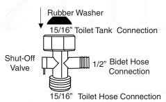
This metal t-adapter has a shut-off valve to limit or cut off cold water to the bidet. It can be used instead of the plastic t-adapter for the cold water connection.
