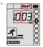
In this example, the user exhaled in endurance mode for 03 seconds at an effort of 5 on level 1.
