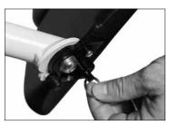
D - Pull ring to disengage lock
