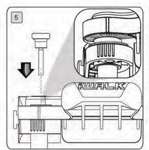
Step 5 - Before attaching the Thigh Support to the Handle, note that there are raised "teeth" on the upper surface of each Thigh Support and on the lower surface of the Handle. These teeth must interlock to prevent rotation of the Thigh Supports when the crutch is in use.
