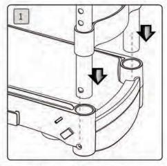
Step 1 - With the Handle facing forward, insert the tubes of the Upper Assembly into the sockets of the Knee Platform. If the hole at the bottom of the Left tube does not align with the hole in the Platform, simply rotate the tube until it does.
