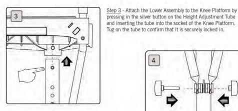
Step 4 - Position the Clamp so it aligns between the ends of the support tubes. You can use gentle pressure to move the Support Tubes while you rotate the Clamp into position. Gently push the support tube ends and align all 4 holes, then insert the Clamp Bolt through the holes. Thread the nut onto the end of the bolt. Do not tighten completely yet.
