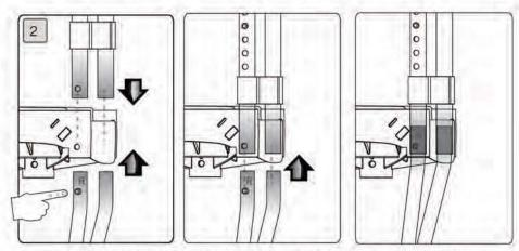
Step 2 - Identify the Right side Support Tube by the small "R" stamped near the top. Press in the small silver button and insert the Support Tube into the bottom of the Knee Platform socket until the button springs into the hole. Make sure the two tubes and the Knee Platform are securely locked together. Next, insert the Left Support Tube.
