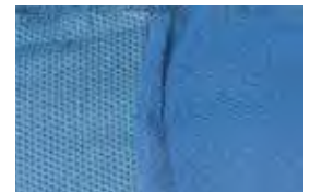
Sonically-sealed seams provide a higher level of protection
