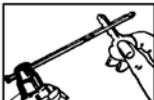
Place a ballpoint pen/key between spray tubes and turn, spreading tubes apart, leaving ballpoint pen/key in place. Remove atomizer tip.
