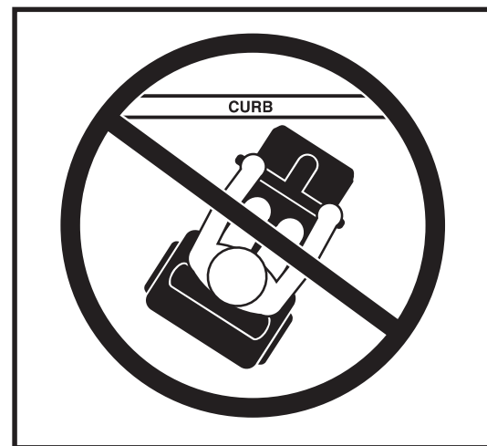
Figure 7. Incorrect Curb Approach
