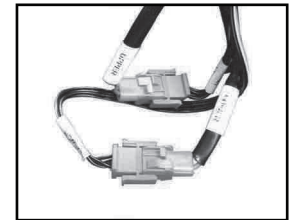
Connect Upper and Lower Cables
