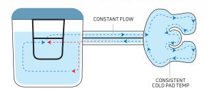
**ICEMAN** with dual pump recirculation technology. The DonJoy® IceMan® features a patented recirculation system that allows water warmed after flowing through the cold pad to be preserved and remixed with cooler ice water at a constant flow rate, providing consistent cool water distribution throughout the cold pad.
