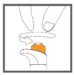
Remove the battery cover by gently twisting it anti-clockwise. It will gradually unscrew from its fixture.
