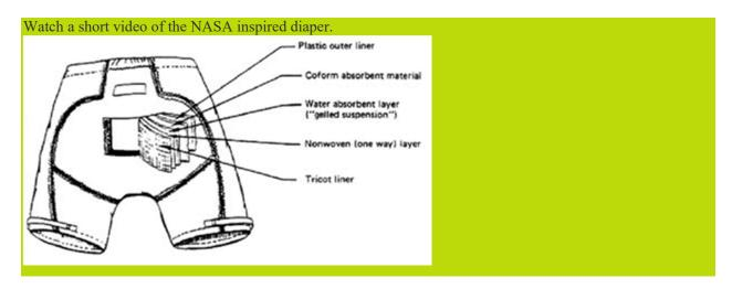
The adult-sized diaper with extra absorption material is used because astronauts cannot remove their spacesuits during long operations. Three MAGs are given during space shuttle missions, one for during launch, reentry, and a spare in case reentry needs to be tried again.
