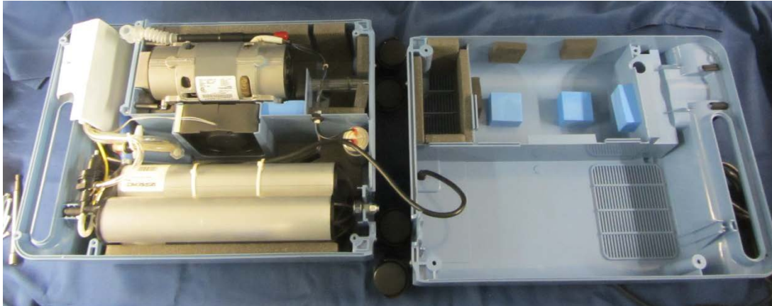
Figure 8-4: EVERFLO REPAIR POSITION
