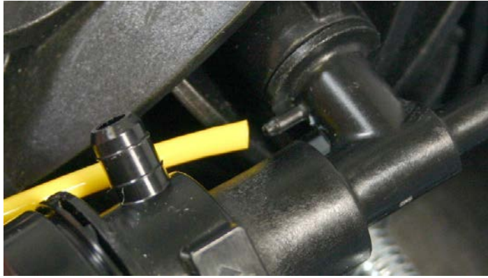
Figure 8-11: PRESSURE LINE REMOVAL
