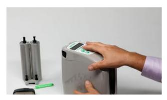
2. Turn unit upside down, and place on soft surface. Remove screws and bottom cover.
