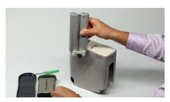
2. Gently push until sieve bed replacement is fully seated, flush with bottom surface. Replace bottom cover and secure screws.
