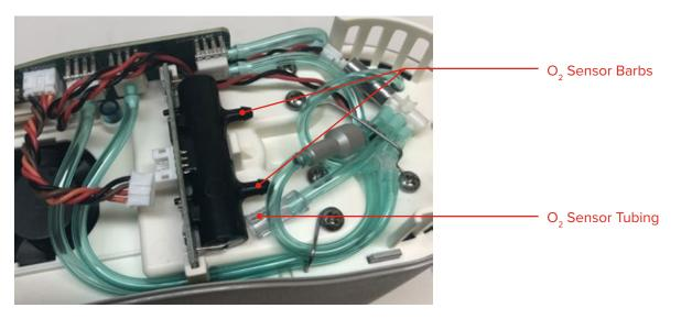
5. With one hand, pull back on the locking tab located on the top separator plate (508538). With the other hand, pull the O2 sensor (508419) up and remove.
