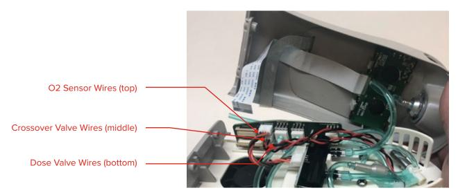
7. Using pliers, carefully remove the tubing that connects to the product tank pressure sensor and dose tank pressure sensor on the PC board (508552). Also remove both tubing pieces from the inspiratory sensor on the PC Board (508552).
