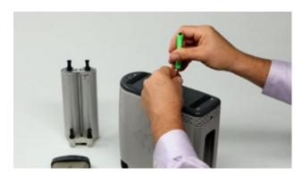
3. Pull upward on the Pull String Loop while holding the device down to remove sieve bed assembly.
