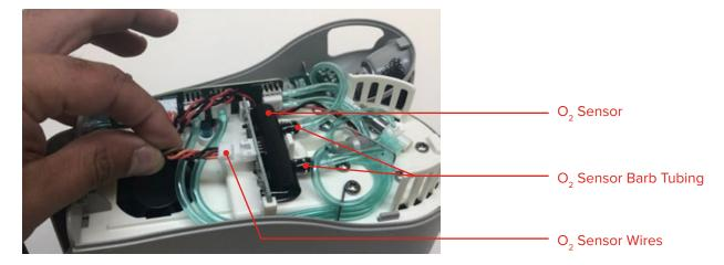
4. Disconnect the tubing from both barbs on the O2 sensor (508419).
