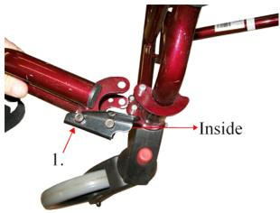
2. Line up the holes on the footrest with the pins on the wheelchair. Let the footrest slide down over the pins
