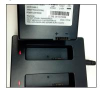
6. Once the external power cartridge is inserted into the charger, it will begin charging. The battery status LED on the charger in front of the external power cartridge will be illuminated to indicate the status of the charging sequence.
