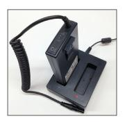
6. The charge will also be indicated by the built-in gauge on top of the external power cartridge. The gauge has four lights (25%-100%) to indicate the level of the charge. While charging a fully discharged external power cartridge, the 25% LED will blink until 25% capacity is reached. The LED will then turn solid and the LED that indicated 50% will blink until 50% capacity is reached. This process will continue until the power cartridge reaches its capacity.
