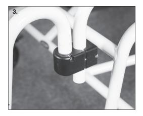
**4.** If the large head support was ordered, remove acorn nut and clamp from headrest assembly.
