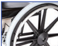
P13857 24" PVC Handrims (replaces standard handrims, pair)
