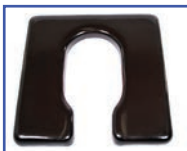
P61117 20"Wx20"D Ensolite® 1" foam Front/Rear Open Seat A-4.5"xB-7.75" opening
