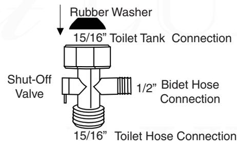
This metal t-adaptor has a shut-off valve to limit or cut off cold water to the bidet. It can be used instead of the plastic t-adaptor for the cold water connection.
