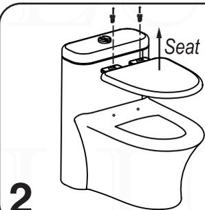
Remove the seat by unscrewing the seat.
