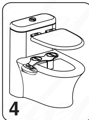
**4** Bidet should now be aligned with the coupling holes.
