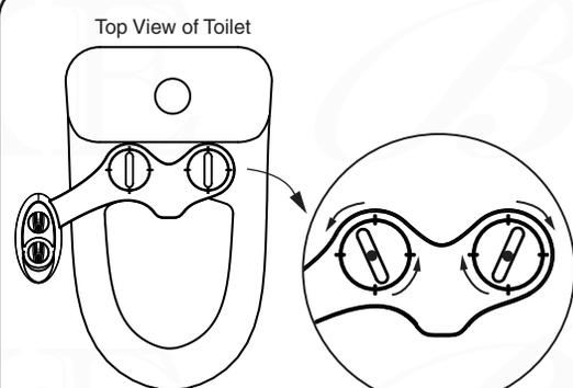
Place the bidet on the toilet. Plates may be adjusted depending on where the two holes in the back of the toilet are.
