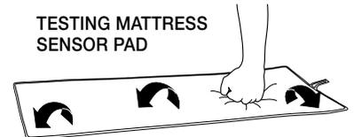
**WARNING** To reduce the risk of serious injury or death, **ALWAYS** follow these steps after putting the sensor pad in place and before leaving resident unattended (see instructions below). Do not use any alarm or sensor pad that does not alarm each time it is tested.
