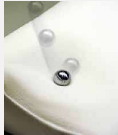
The material responds only slightly to energy applied to it, clearly demonstrating the pressure relieving effect of the visco-elastic foam.
