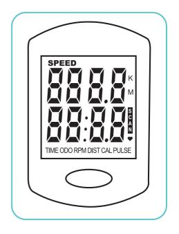
**CAL:** Shows the number of calories burned (O.OO-999.9). (This mode states an approximate value. The actual calorie consumption depends on the condition of the person).
