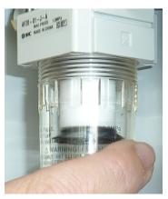
Fig. 4 - 9 Screwing the pressure filter housing in place
