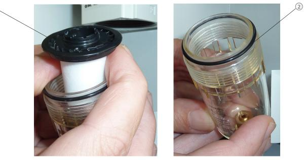
Fig. 4 - 5 Filter element holder removed
