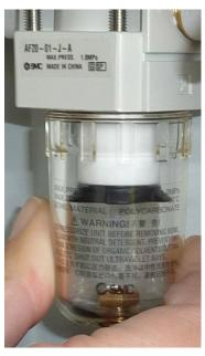
Fig. 4 - 3 Unscrewing the pressure filter housing
