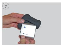
• The protective cushion can be pulled back and up off the handpiece handle to clean the handpiece.
