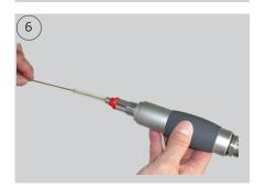
• Clean the guide tube with a brush in order to ensure perfect projectile movement.
