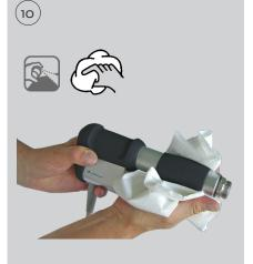
• Clean the shaft, the transmitter (including firmly seated sealing rings) and the transmitter screw cap with an alcohol-based disinfectant. These are reused after cleaning.
