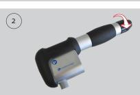
• Unscrew the transmitter screw cap from the handpiece.
