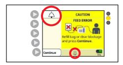
The alarms cannot be permanently silenced or muted. However, by pressing the Silence Alarm button, the alarm audio will be temporarily silenced for two minutes. After two minutes, the alarm audio will restart. To re-engage the audio alarm before the two minutes is up, press the Bell button. This will end the temporary audio pause, and restart the audible alarm.
