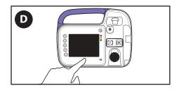
D. If alarm continues after replacing Kangaroo OMNI™ Feeding Set, press **Power Off** to stop operation and use a different Kangaroo OMNI™ Enteral Feeding Pump.
