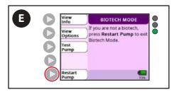
E. Press **Restart Pump** button to save the settings and exit Biotech mode. If a user attempts to modify any settings, a Settings Locked reminder screen will be displayed. The Lock Settings feature can only be disabled by entering Biotech Mode and switching Lock Settings to Off.
