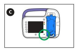
C. Confirm the green Power Indicator Light is on to ensure Kangaroo OMNI™ Enteral Feeding Pump is receiving power.
