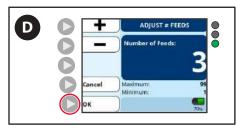
D. Press **OK** to save the settings and return to the **Adjust Feed** screen.
