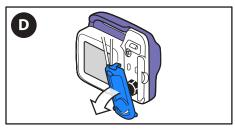
D. If alarm continues, **turn off pump** and **Remove** the cassette from Kangaroo OMNI™ Enteral Feeding Pump.
