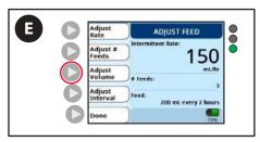
E. Press the **Adjust Volume** button to set the Feed volume.
