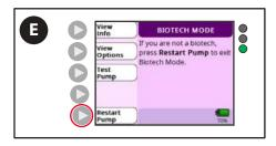
E. Press **Restart Pump** button to exit Biotech mode and return to normal operating mode.
