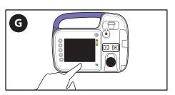
G. If alarm continues after replacing Kangaroo OMNI™ Feeding Set, press **Power Off** to stop operation and use a different Kangaroo OMNI™ Enteral Feeding Pump.
