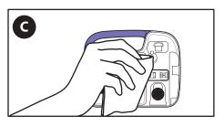
C. **Clean and dry** the Kangaroo OMNI™ Enteral Feeding Pump valve actuator.
