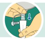
Step 1: Gently insert the ridged part of the end of the tap into the wider section of the adaptor with one hand while holding the base.
