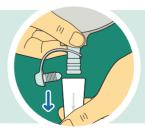
Step 2: To remove, pull out Connector with one hand while holding base of tap with the other hand.
