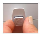
Insert the Patient Interrupt Switch Hook Cover to cover the Hook Screw Hole.
