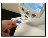
Insert the Patient Data Card (with the gold chip facing up) to be erased into the Patient Data Card port located on the front of the traction unit.
