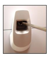
Place the Patient Interrupt Switch Hook over the Screw Hole and tighten the Hook Screw in place.
