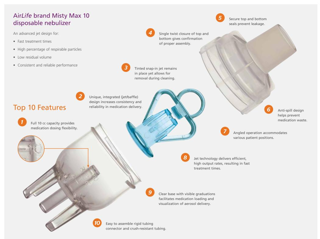
Delivering fast and effective treatment, more efficiently. Accommodating all types of patients in all types of situations. These were the forces behind the development of the Misty Max 10 nebulizer. Featuring a new type of jet design, the Misty Max 10 nebulizer can speed up treatment and help ensure consistent medication delivery while offering you more flexibility in treatment options.
