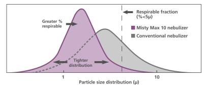
Particle size is an important characteristic of nebulizer performance. The Misty Max 10 nebulizer provides fine particles with a tighter distribution.
