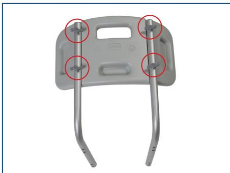
4. Attach backrest to the seat by aligning holes on "L" shaped frame supports with the holes on the leg sections. Secure in place using the longer thumb screws, making sure to pay attention to the "rear" of the seat marked on the bottom of the chair.
