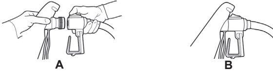
Figure 3 – Attaching the Collection Bag
