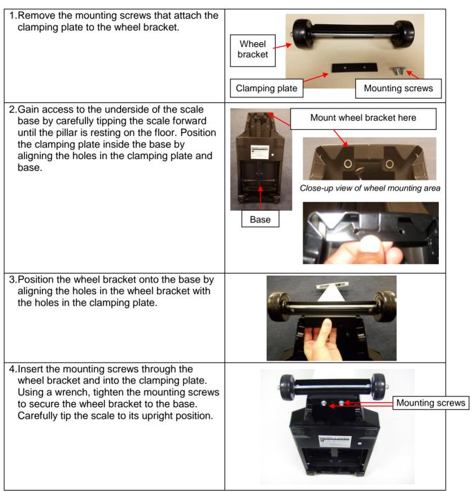
To transport the scale, tip the pillar backwards until the scale is resting on the wheel bracket. Carefully move the scale to its new location.
