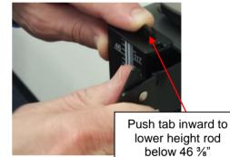
To lower height rod below 46 %", push the tab at the top of the height rod and gently lower the headpiece.
