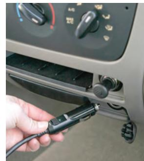
and securely remain in place. The Cigarette Lighter Adapter comes with a slide switch pre-adjusted to the narrow position. This will fit most automobile cigarette lighter sockets. If the Cigarette Lighter Adapter is loose in the socket, adjust the switch to the "wide" position.
