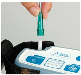
5. Connect the nasal cannula securely to the cannula nozzle fitting on the unit but DO NOT put it in your nose until after the unit has been powered on. Breathing through the cannula during start-up may prevent the system from starting.
