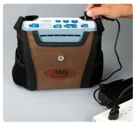
2. Charge the unit before the first use. To charge the unit, connect the AC Adapter to the unit as shown in the picture and then connect the AC Charger to an electrical outlet.
