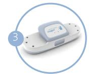
Slide the charger onto the Inogen One G3 Battery by clicking and locking into the charger.
